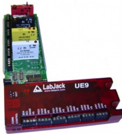
Figure 3: RB12 w/ modules connected to UE9
