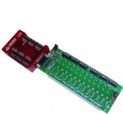
Figure 2: RB12 connected to U3
